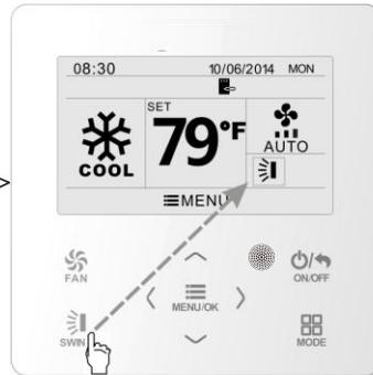
Press SWING button to turn on or turn off simple up&down swing and fixed-angle up&down swing
