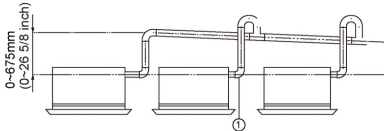
① - drainage pipes assembled by T-shaped joints
