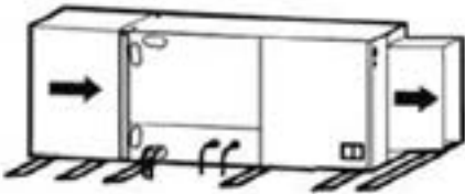
Horizontal Right Configuration - Must Relocate Drain Pan
