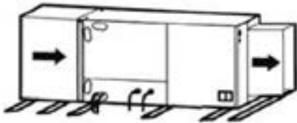
Horizontal Right Configuration - Must Relocate Drain Pan
