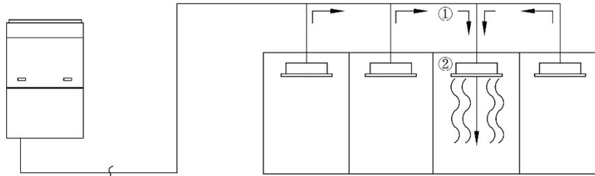
① Flow direction of refrigerant leakage.
