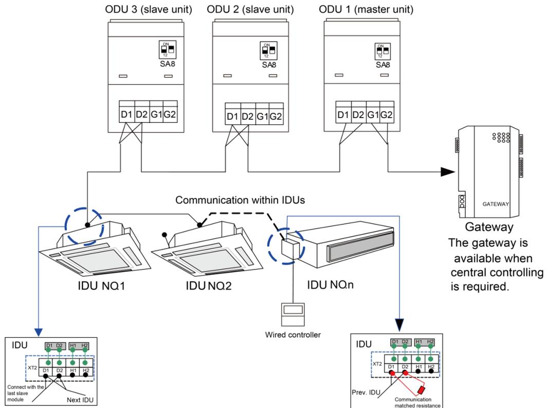
Fig.52 Connection of modular unit
