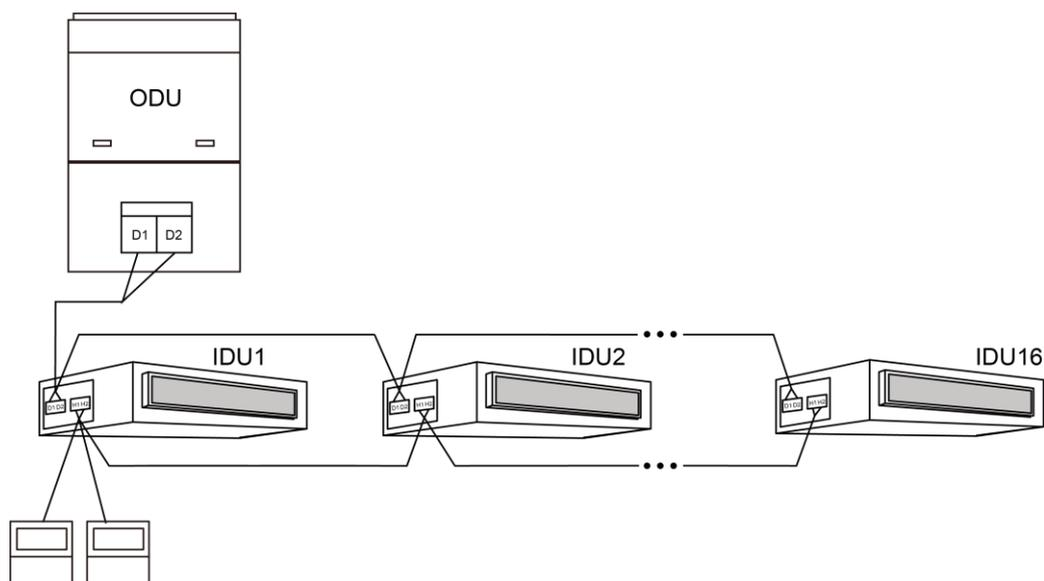
Fig.56 Two wired controllers control multiple IDUs
