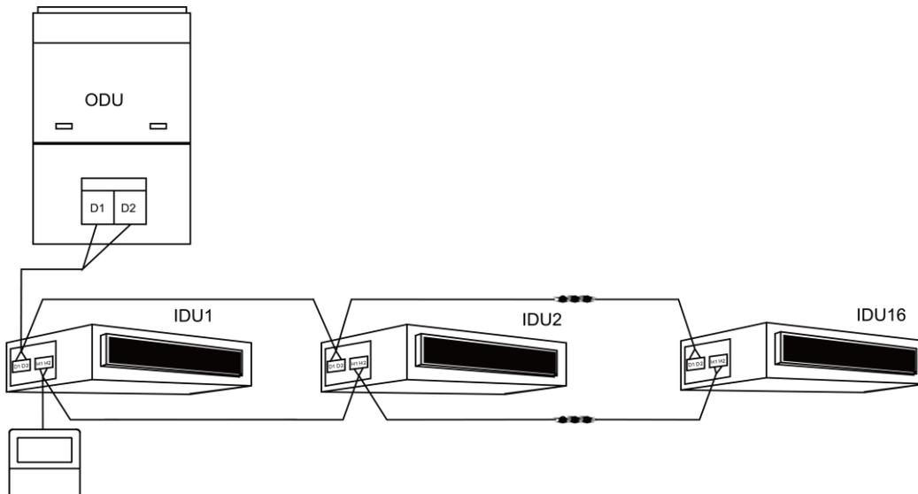
Fig.55 one wired controller controls multiple IDUs
