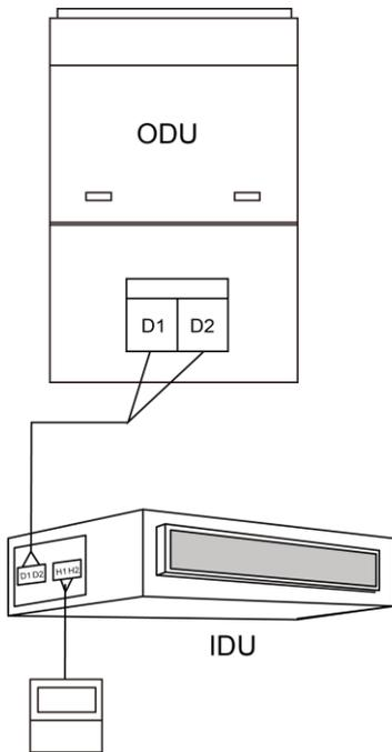
Fig.53 one wired controller controls one IDU
