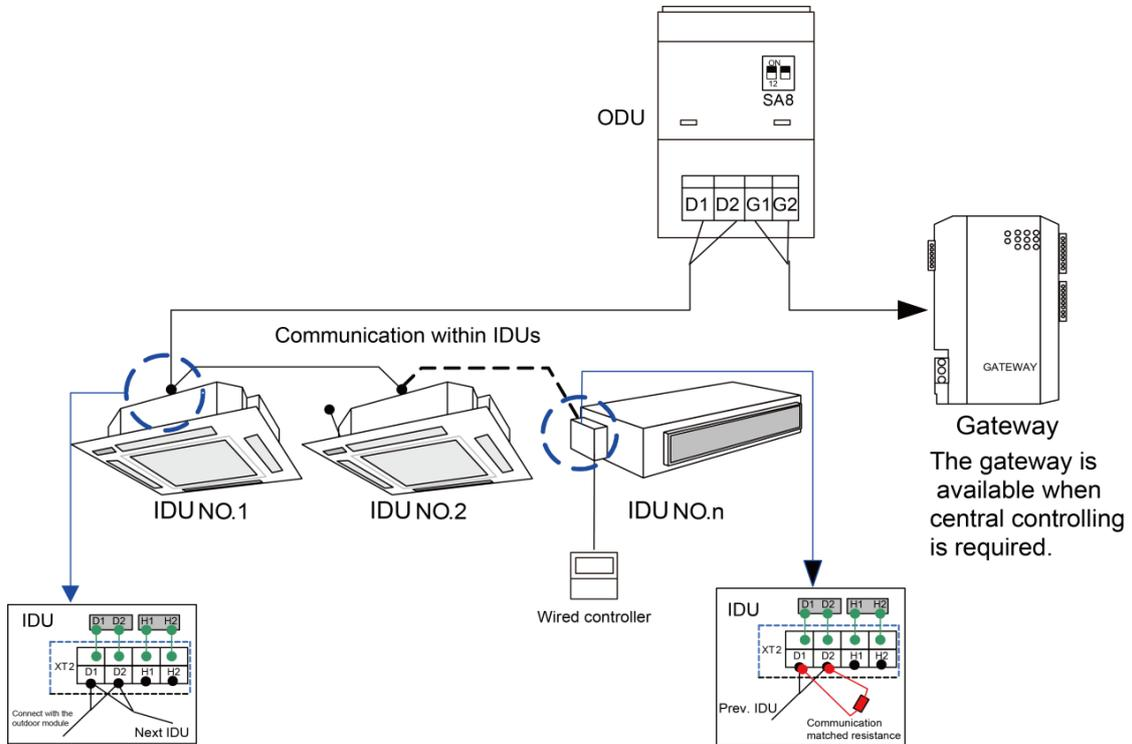
Fig.51 Connection of single unit
