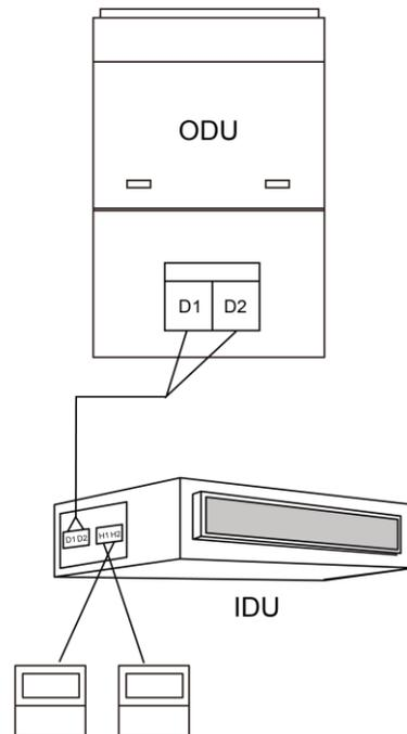
Fig.54 Two wired controllers controls one IDU
