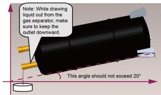
Use a glass container to hold the liquid. Check liquid impurities and colours and block the container for further factory inspection.
