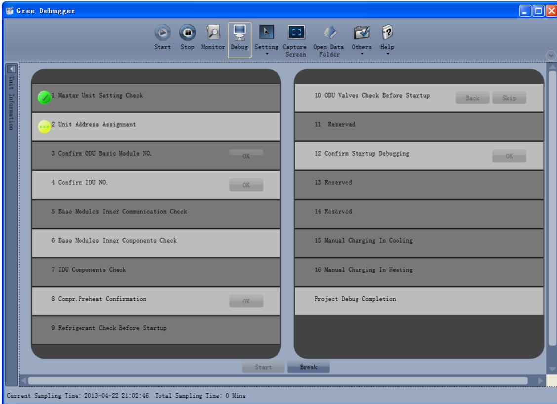
For the phase with "OK" displayed, a manual confirmation is required for entering the next commissioning step. Click "🟡" to display relevant information detected on this phase, which provides references for selection. Click "Close" to close the information (the number of commissioning units is displayed in "3 Confirm ODU Basic Module NO." and "4 Confirm IDU NO."; the preheating period is displayed in "8 Compressor. Preheat Confirmation").
