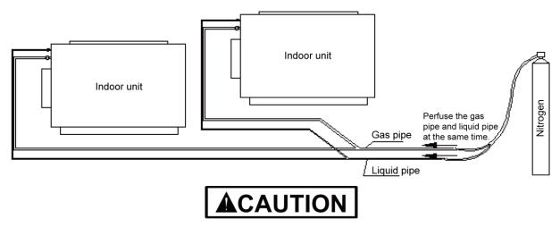
Before performing the air-tightness test, do not conduct insulation or wrapping at the welding joints, Otherwise, leak source cannot be detected quickly.
