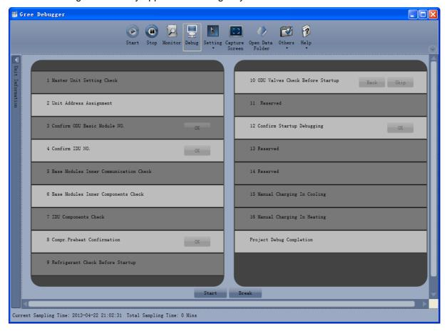
Click "Start" to enter the commissioning function and the software automatically performs commissioning. " indicates that commissioning is being performed on the phase and " indicates that commissioning is passed on the phase.
