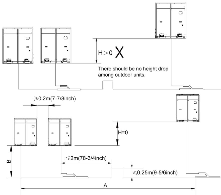
**NOTE:** When the distance between outdoor units exceeds 2m (6-5/9feet), U-type oil trap should be added at low-pressure gas pipe.  $A+B \leq 10\text{m}$  (32-3/4feet).
