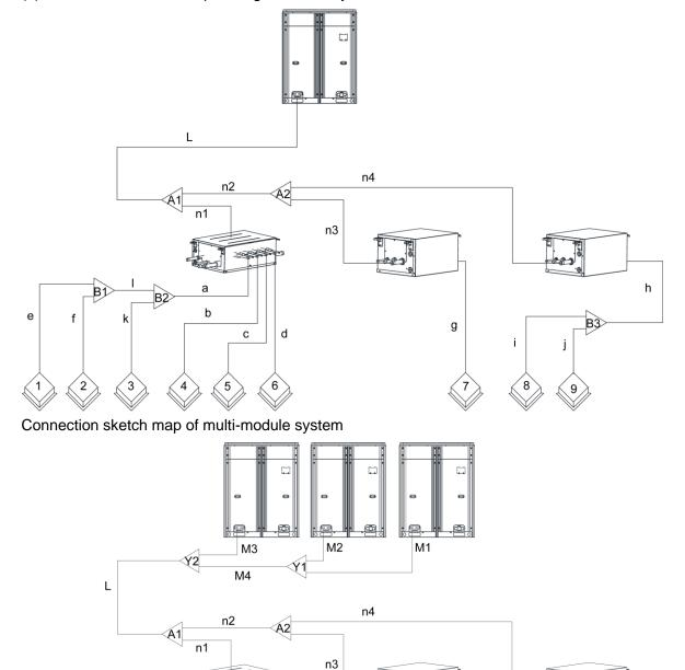
(2) Select appropriate pipe between outdoor unit and the first indoor branch ("L") as per the pipe size of outdoor unit. Pipe size of basic outdoor module is shown as follows:
