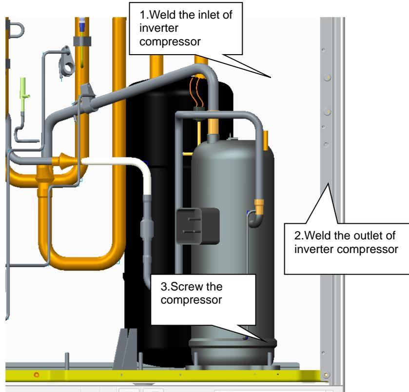
For compressors of GMV-Q120WM/B-F(U) units, make sure the new compressors are consistent with the faulty ones in model. If both compressors need replacement, make sure corresponding position and wiring are correct. You are advised to replace them one after another.
