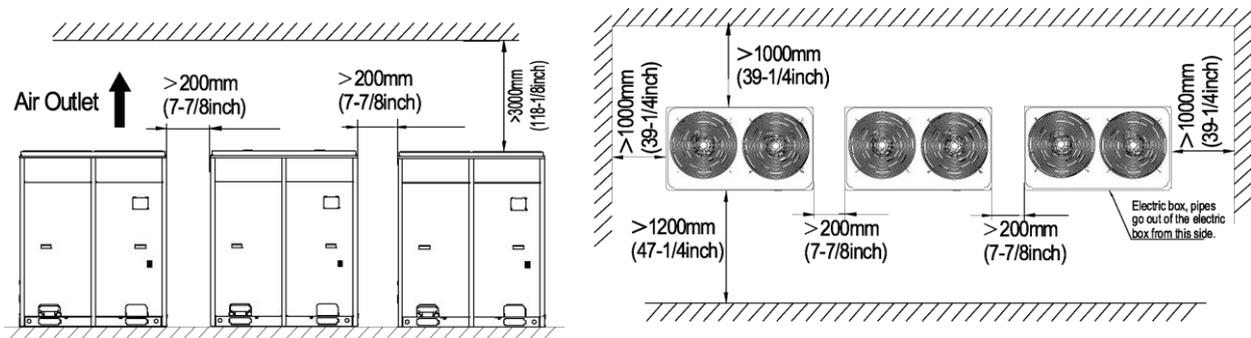
(2) When there is wall (or similar obstruction) above the unit, keep the distance between the unit top and the wall at least 3000mm (118-1/8inch) or above. When the unit is located in a totally open space with no obstructions in four directions, keep the distance between the unit top and wall at least 1500mm (59inch) or above (See Fig.1). When space is limited within 1500mm
