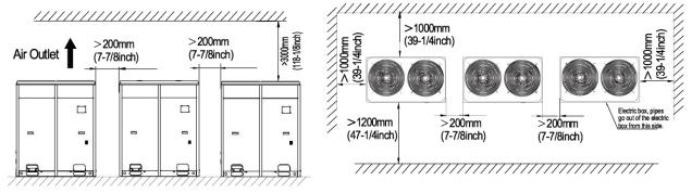
(2) When there is wall (or similar obstruction) above the unit, keep the distance between the unit top and the wall at least 3000mm (118-1/8inch) or above. When the unit is located in a totally open space with no obstructions in four directions, keep the distance between the unit top and wall at least 1500mm (59inch) or above (See Fig.1). When space is limited within 1500mm
