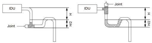
(13) During condensate water pipe installation, ensure a distance above 500mm (19.7inch.) between the pipe and the electric box of the unit for maintenance. In a case when the space is not enough, the final piping way must be determined by the technical personnel.
