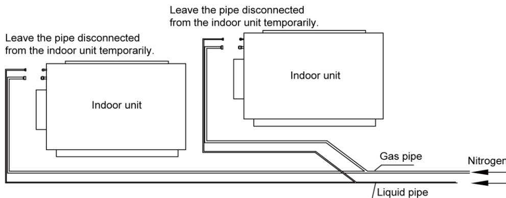
Perform an air-tightness test and a vacuum test to the entire refrigerant pipe system after the construction is finished.
