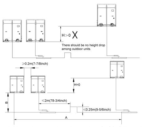
**NOTE:** When the distance between outdoor units exceeds 2m (6-5/9feet), U-type oil trap should be added at low-pressure gas pipe. A+B≤10m (32-3/4feet).
