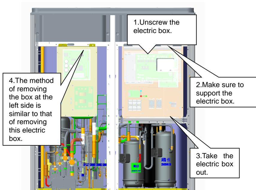
For GMV5 HR series, only GMV-Q120WM/B-F(U) units are configured with the left electric box, which contains mainly the drive of the compressor E405DHD-38A2YG. After the box is removed, take care with the removal of electric parts' lines. DO NOT pull the lines with excessive force; or they may be broken. The removed electric box must be protected for dustproof and waterproof purposes.
