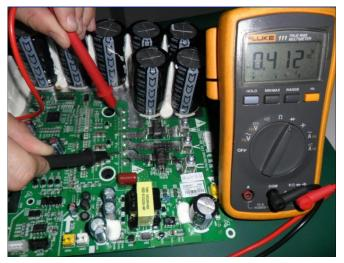
(6) As shown in the figure below, put the black test probe to pad V (YE) and the red test probe to
