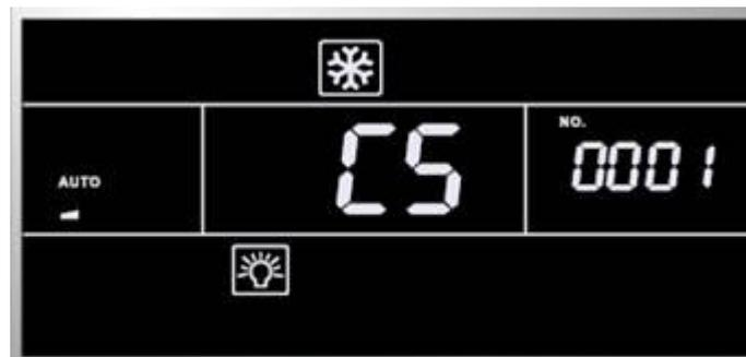
If this fault occurs, the number of the new AP1 is identical to that of a unit within the network. Manually change it to the original number of the faulty AP1 or a unique number. There are three methods to change project number:
