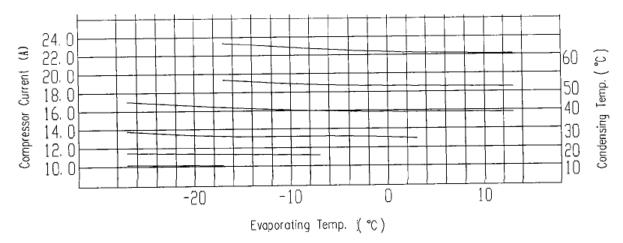
The figure below shows current curves that change with evaporating temperature and condensing temperature while the compressor works at 90 Hz.
