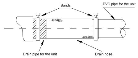
e) Apply insulation materials to the condensate water pipe joints to prevent dewing. d. Insulation for connection between the drain pipe and that of the IDU is shown in the following figure.
