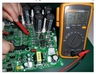
(5) As shown in the figure below, put the black test probe to pad U (BL) and the red test probe to pad NU (make sure the moisture proof tape is removed). In normal cases, the multimeter should read 0.39±0.3 V. If it is "0" or infinitely great, the IPM module is faulty.
