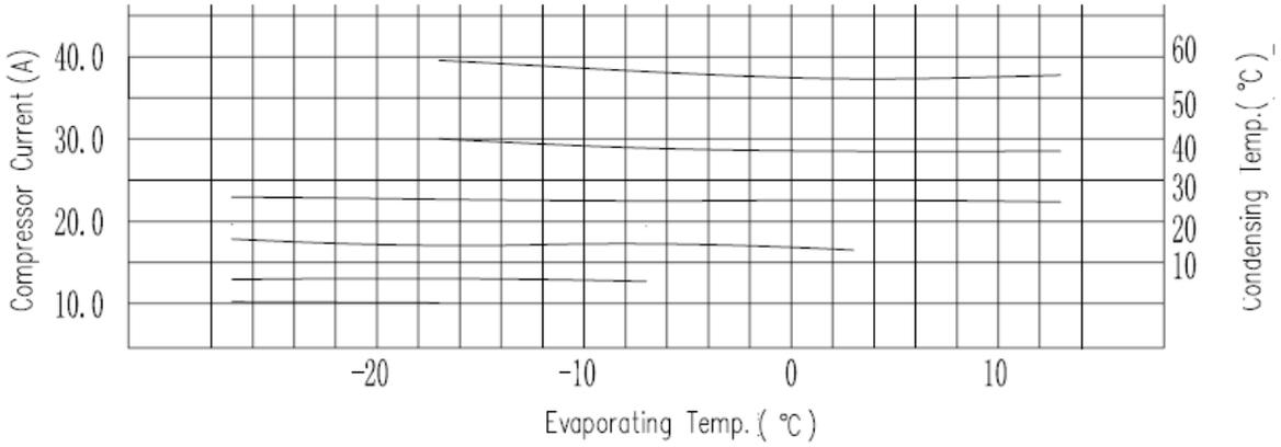
The figure below shows current curves that change with evaporating temperature and condensing temperature while the compressors work at 60 Hz.
