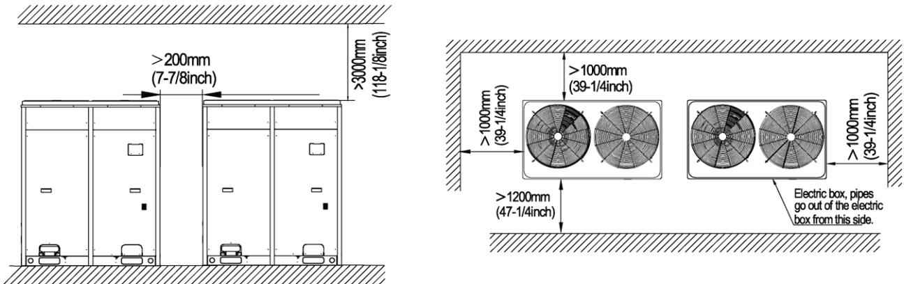
3) Installation space requirements for triple-module unit
