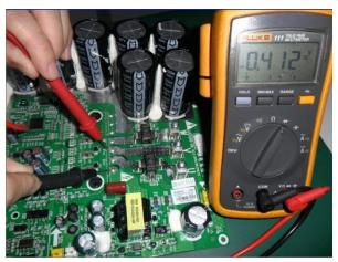
(4) As shown in the figure below, put the black test probe to pad P and the red test probe to pad W (RD) (make sure the moisture proof tape is removed). In normal cases, the multimeter should read 0.39±0.3 V. If it is "0" or infinitely great, the IPM module is faulty.
