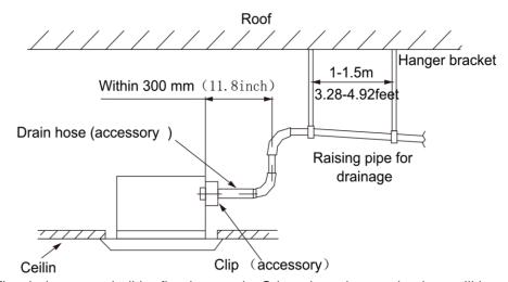
c) The drain pump shall be fixed securely. Otherwise, abnormal noises will be generated.
