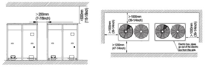
3) Installation space requirements for triple-module unit
