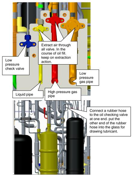
**Note:** Lubricant is of great importance to the normal running of compressors. You should follow Gree's requirement to add qualified lubricant of the specified trademark and ensure properness of fill
