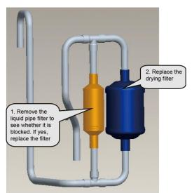
For other pipeline parts, clear them based on actual situation. If you do not replace the parts immediately, make sure to block the pipes with tapes, preventing air moistures and impurities from contaminating them.
