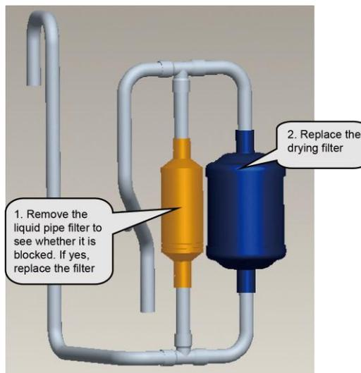
For other pipeline parts, clear them based on actual situation. If you do not replace the parts immediately, make sure to block the pipes with tapes, preventing air moistures and impurities from contaminating them.
