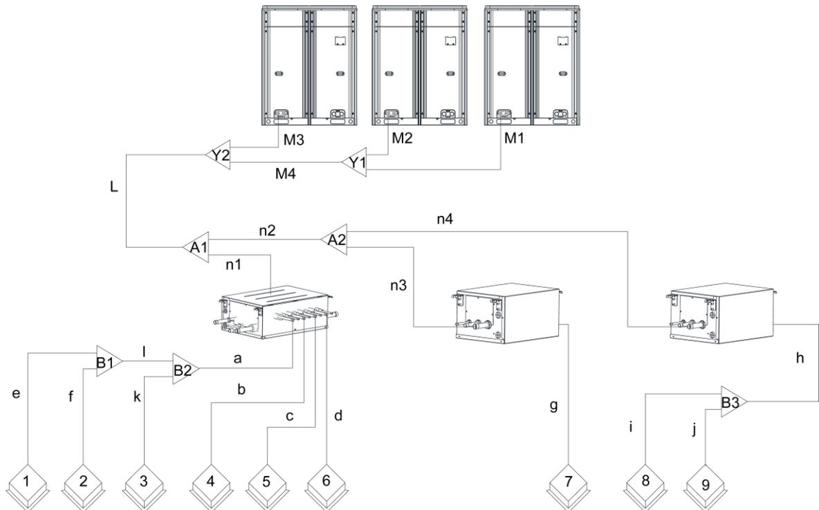
(2) Select appropriate pipe between outdoor unit and the first indoor branch (“L”) as per the pipe size of outdoor unit. Pipe size of basic outdoor module is shown as follows:
