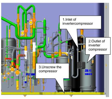
After the compressor and oil separator are removed, check oil quality. If oils are contaminated, replace the compressor, oil separator, and gas/liquid separator. If oil changes to black, check oils of other modular units. The check procedure is similar to the preceding.
