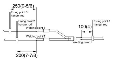
Branches of a manifold must be laid parallel and cannot be wrapped in superimposed mode.
