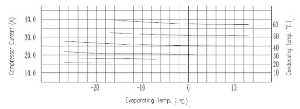
The figure below shows current curves that change with evaporating temperature and condensing temperature while the compressors work at 90 Hz.
