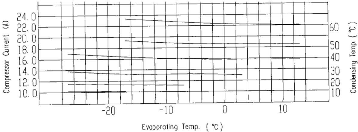
The figure below shows current curves that change with evaporating temperature and condensing temperature while the compressor works at 90 Hz.
