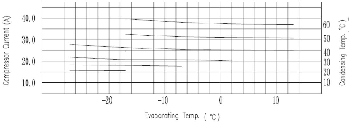
The figure below shows current curves that change with evaporating temperature and condensing temperature while the compressors work at 90 Hz.
