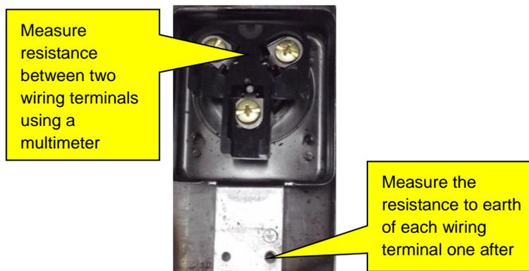
Measure the resistance to earth of each wiring terminal. The value should be 10 MΩ. If not, the compressor has an internal fault.
