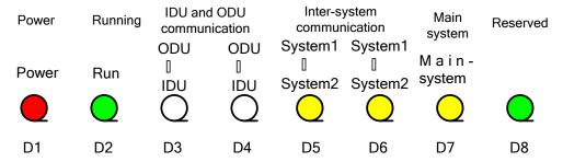
If the LEDs flash, the ODU and IDUs normally communicate; if the LEDs are steadily on, communication is faulty. Check communication lines connecting the ODU and IDUs.
