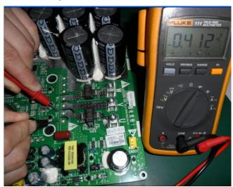
(3) As shown in the figure below, put the black test probe to pad P and the red test probe to pad V (YE) (make sure the moisture proof tape is removed). In normal cases, the multimeter should read 0.39±0.3 V. If it is "0" or infinitely great, the IPM module is faulty.
