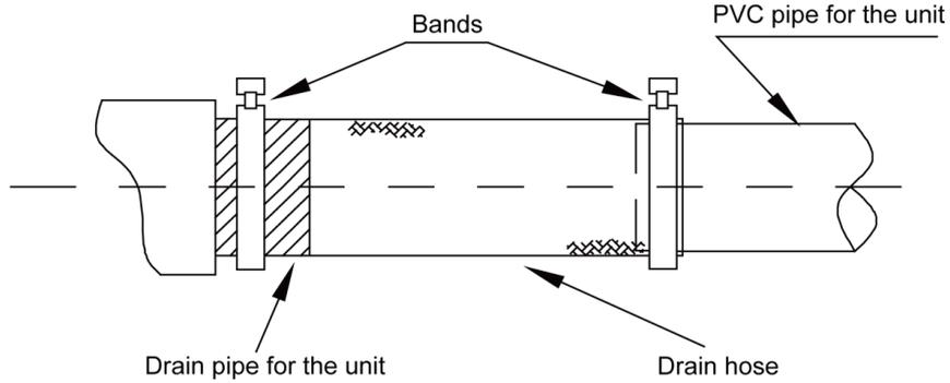
e) Apply insulation materials to the condensate water pipe joints to prevent dewing. Insulation for connection between the drain pipe and that of the IDU is shown in the following figure.
