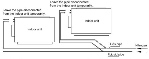
Perform an air-tightness test and a vacuum test to the entire refrigerant pipe system after the construction is finished.
