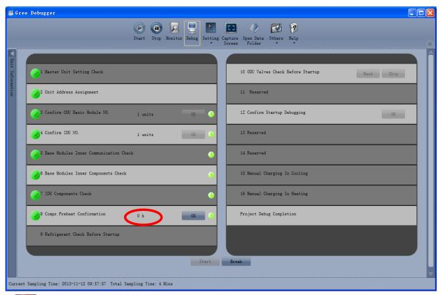
"indicates that commissioning is not passed on the phase and troubleshooting is required (after troubleshooting, the unit automatically enters the next step if no "OK" exists or click "OK" to enter the next step). Click "Im" to display relevant information detected on this phase, which provides references for troubleshooting. Click "Close" to close the information.
