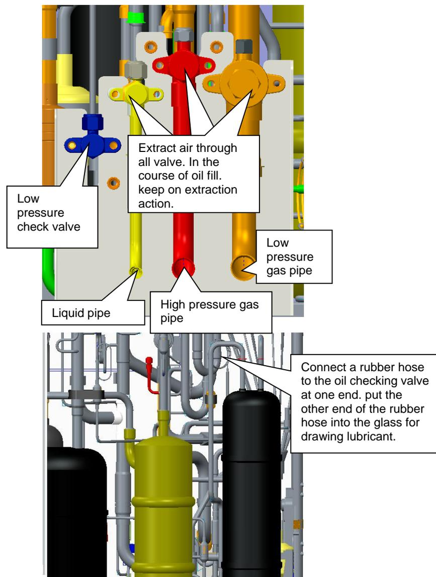
**Note:** Lubricant is of great importance to the normal running of compressors. You should follow Gree's requirement to add qualified lubricant of the specified trademark and ensure properness of fill
