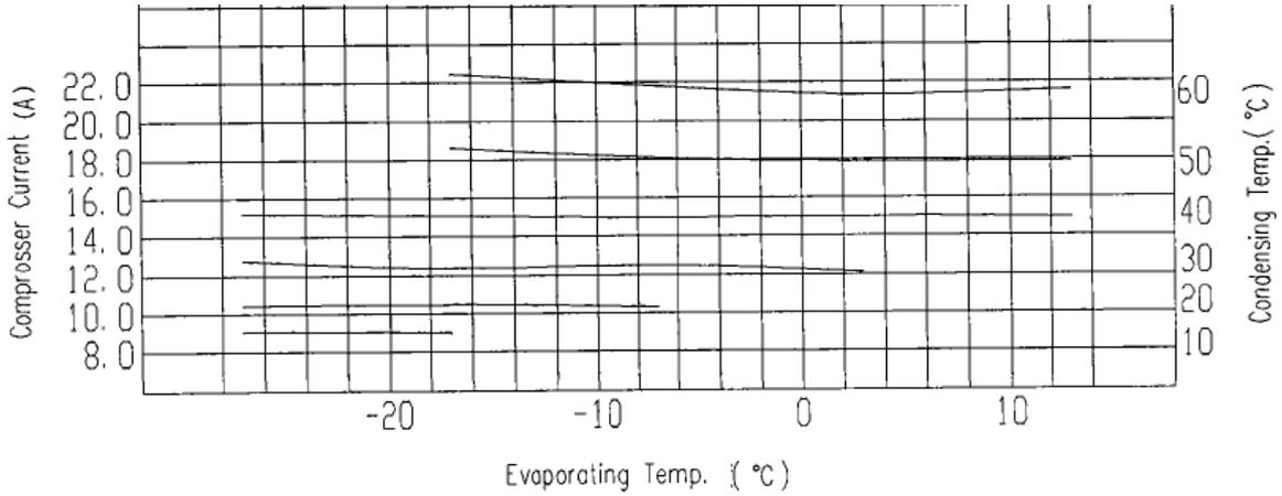
The figure below shows current curves that change with evaporating temperature and condensing temperature while the compressor works at 60 Hz.
