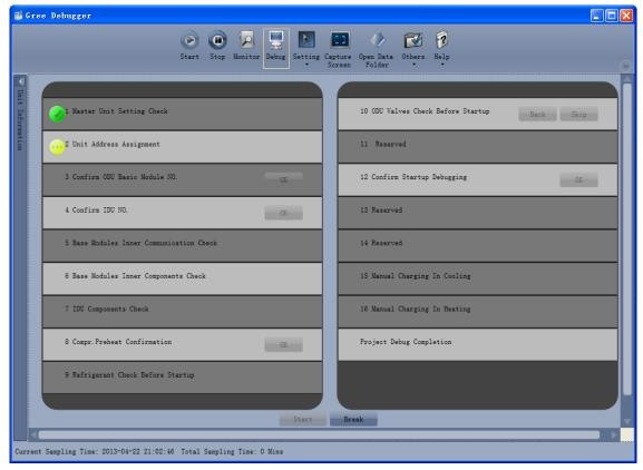
For the phase with "OK" displayed, a manual confirmation is required for entering the next commissioning step. Click "U" to display relevant information detected on this phase, which provides references for selection. Click "Close" to close the information (the number of commissioning units is displayed in "3 Confirm ODU Basic Module NO." and "4 Confirm IDU NO."; the preheating period is displayed in "8 Compressor. Preheat Confirmation").
