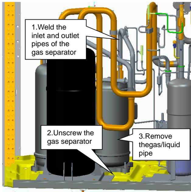
After the gas separator is taken out, check whether it contains impurities. The check procedure is as follows:
