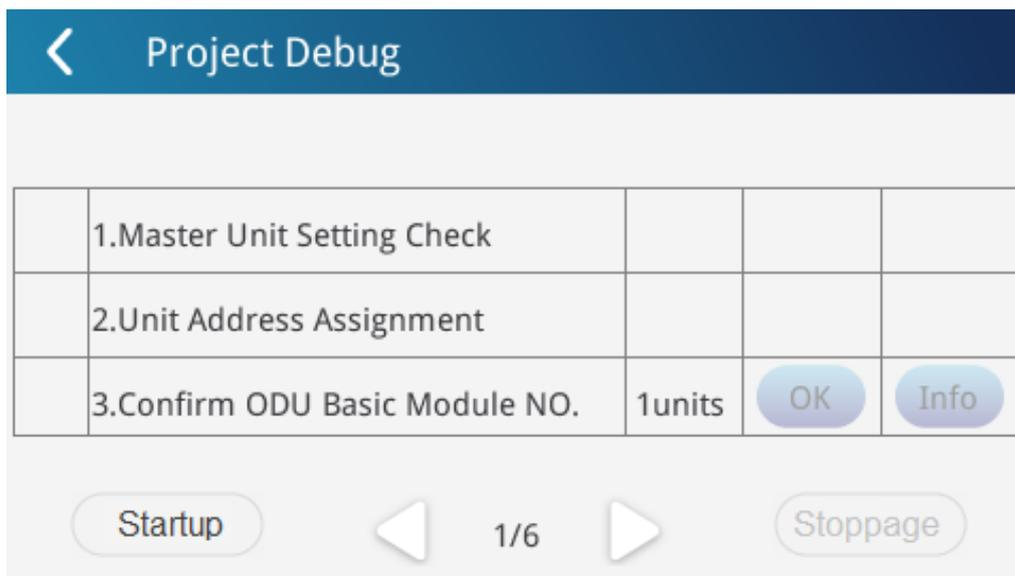
Step 5: Once it entered the engineering debugging, Portable Commissioning Tool will display current progress of engineering debugging (step#). As for step 3, 4, 8 and 12,
