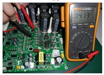
(7) As shown in the figure below, put the black test probe to pad W (RD) and the red test probe to pad NW (make sure the moisture proof tape is removed). In normal cases, the multimeter should read 0.39±0.3 V. If it is "0" or infinitely great, the IPM module is faulty.
