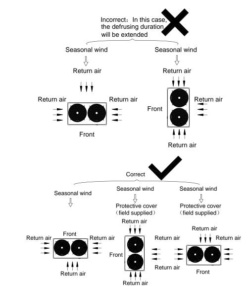
(4) Anti-monsoon installation requirements for unit connecting exhaust duct:
