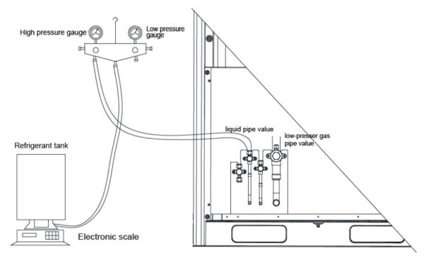
Step 5: Turn on the valve of the high pressure gauge (while keep the valve of the high pressure gauge turned off) and then perfuse refrigerant to the system. Record the change of weight of the refrigerant tank.
