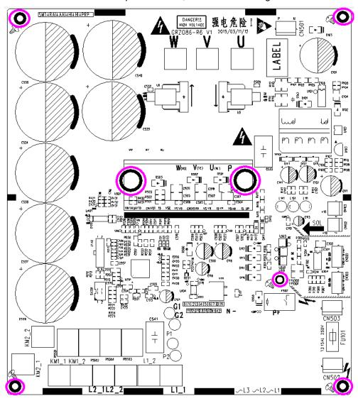
(5) Replace the compressor drive. Before the replacement, apply some silicone tape onto the IPM module.
