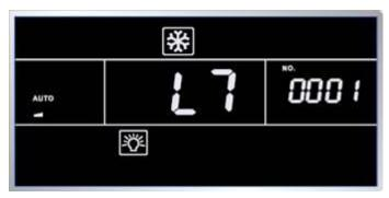
Method 1: If the IDU is configured with wired control, stop the IDU (except for lock mode) and press and hold the "MODE" button for 5 seconds to enter setting mode. After setting, the "Master" icon will be highlighted and the wired control buzzer will beep once.
