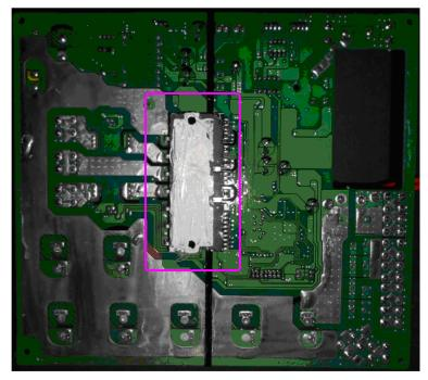
(6) Install a new compressor drive, screw and wire it.
