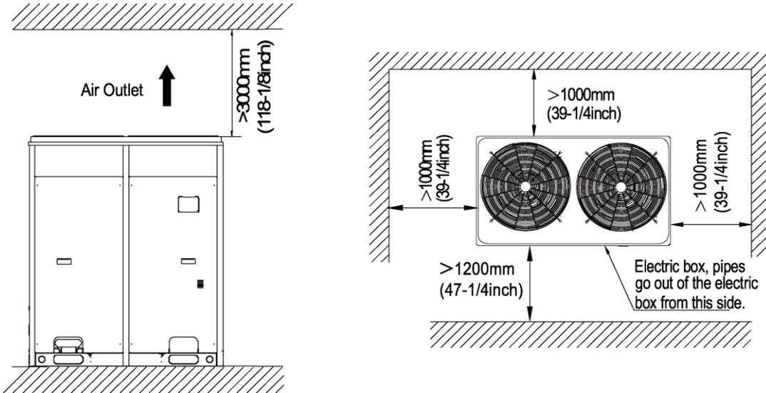
2) Installation space requirements for the dual-module unit
