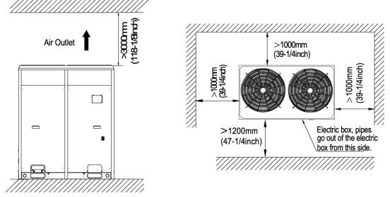
2) Installation space requirements for the dual-module unit
