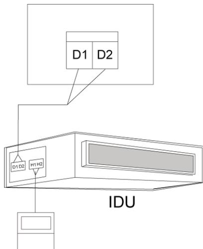
Fig.44 One wired controller controls one IDU
