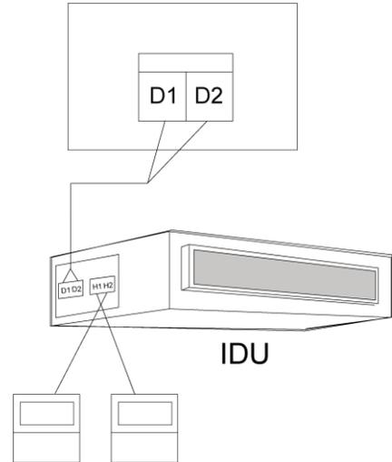
Fig.45 Two wired controllers control one IDU
