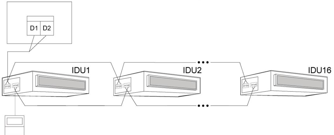
Fig.46 One wired controller controls multiple IDUs
