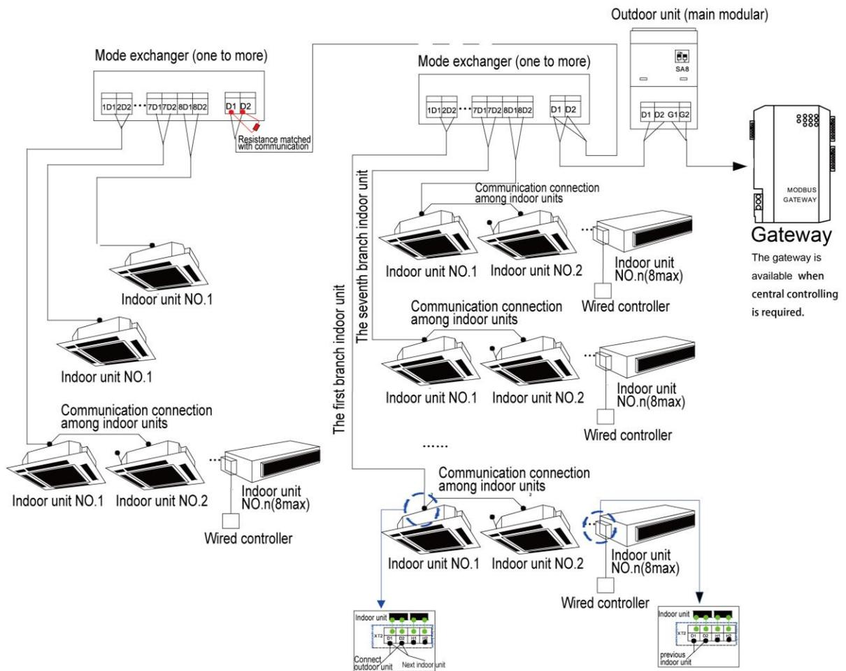
Fig.42 Connection of communication for single-module system and multi-module converter system
