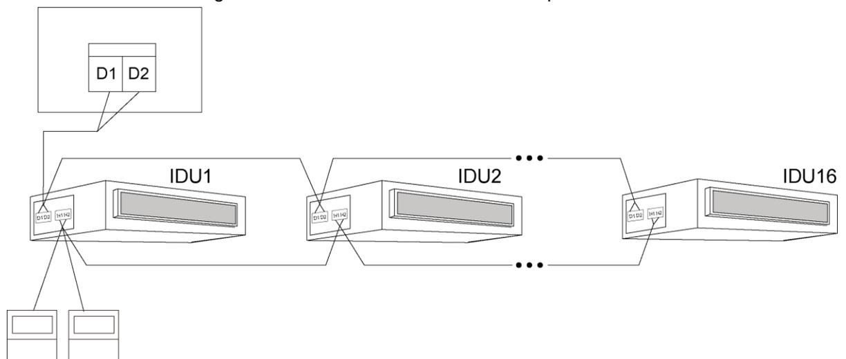
Fig.47 Two wired controllers control multiple IDUs
