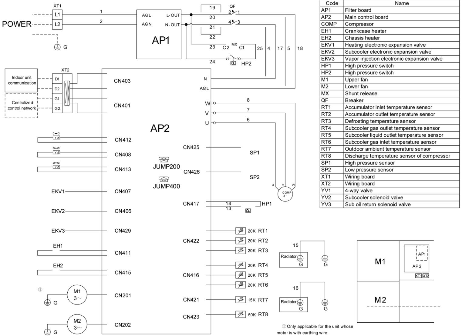
**Note:** Refer to the mark on the unit for the actual circuit diagram.
