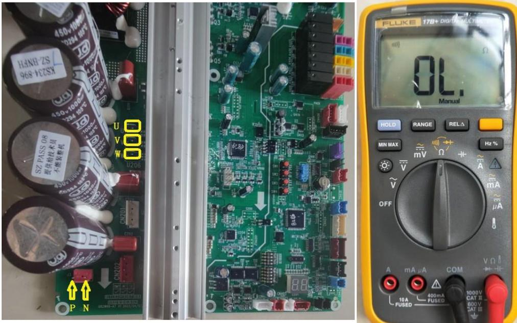
3: Point the black probe to the P needle file and the red probe to the V wiring terminal. In the normal condition, the multimeter will not beep. If it does, the drive board is damaged and needs to be replaced.
