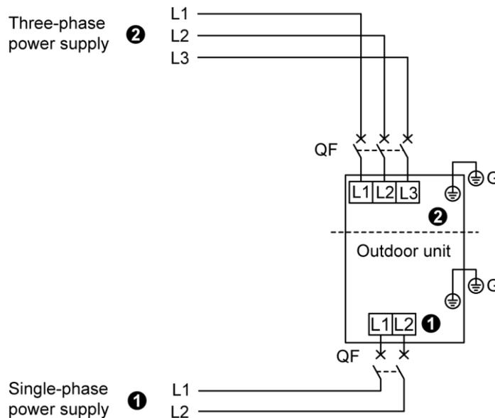
NOTE: For single-phase units, connect wires according to drawing ①; for three-phase units, connect wires according to drawing ②.
