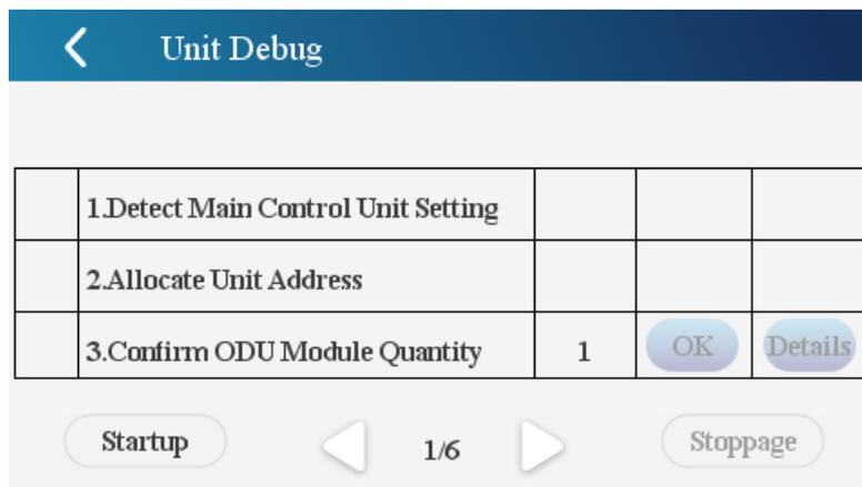
**Step 4:** During commissioning, multi-functional debugger shows the current process (step). In steps 3, 4, 8, and 12, click Confirm to go to the next step. In step 10, click Skip or Back. In steps 3, 4, 5, 6, and 7, you can view the details.
