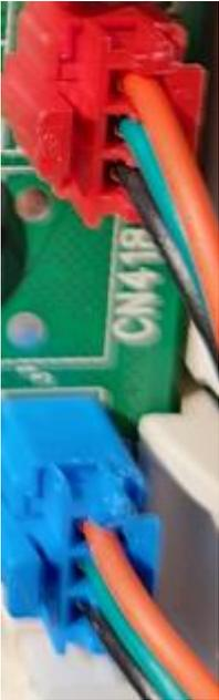
**Black to Orange is the output voltage from the board. 5VDC**
