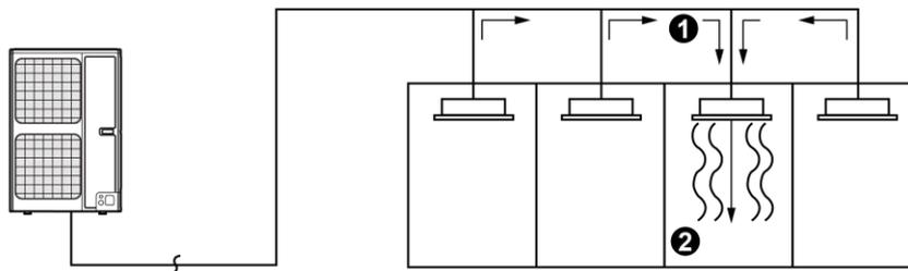
① Flow direction of refrigerant leakage
