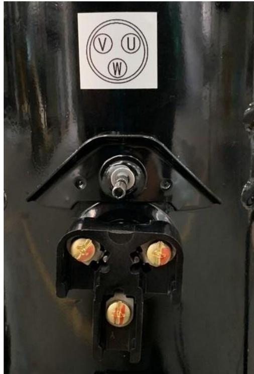
Measure the grounding resistance of each wiring terminal, which should be greater than 10 M $\Omega$ ; otherwise, the compressor has an internal fault.
